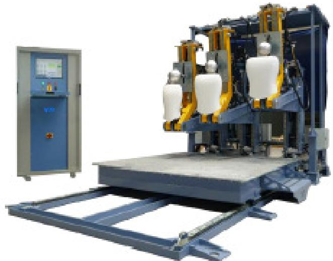
The ranges of the movements can be defined by the customer depending on the range of the seats to be tested. The test is performed automatically, recording the torque-time, force-time and head penetration-time.
